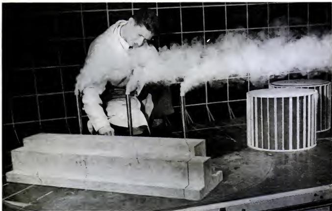
An engineer towers over the "300-ft." stacks of an experimental model of Con Edison's pro-
